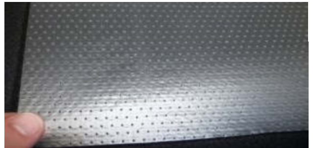
Pic. 7: The perforated release film HP-RF25/110 in a close-up view.
