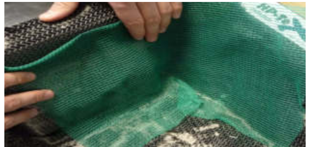
Pic. 8: Adjusting the vacuum mesh HP-IM145/100 .
