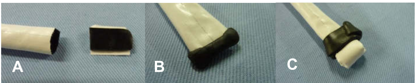
Pic. 14, A-C: MTI ®-hose. Sealing the ends.
