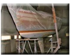
Hull is masked off for further work steps after drying
