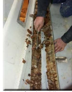
Yielding decking suggests damage to the laminate and this extent becomes after opening recognizable
