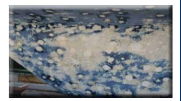
First, the underwater hull was cleaned, degreased and sanded.
