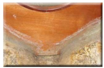
Crack in transition main bulkhead to bilge
