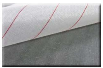
Surface after tearing off the fabric
