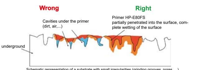
Schematic representation of a substrate with small irregularities (grinding grooves, pores, ...)
