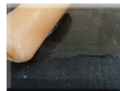
Epoxy resin is distributed with velour roller
