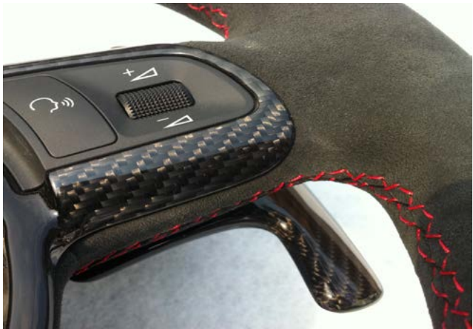
A steering wheel coated with carbon fabric.
