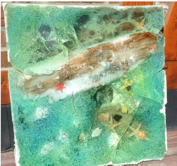
Stress cracks + boiling bubbles
