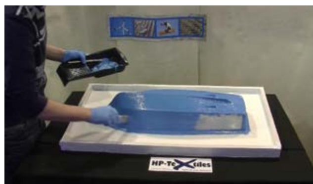
Application of the mould making resin (special colour blue)
