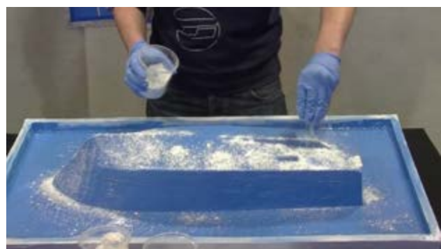
Spreading the dry coupling layer (glass fibre chips and cotton flocks)
