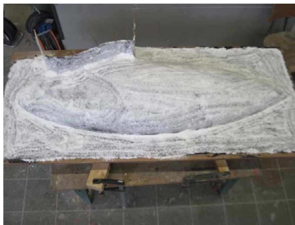
Dry coupling layer of cotton flocks & glass fibre shreds
