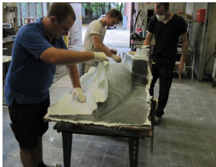
Reinforce back with epoxy resin and carbon/glass
