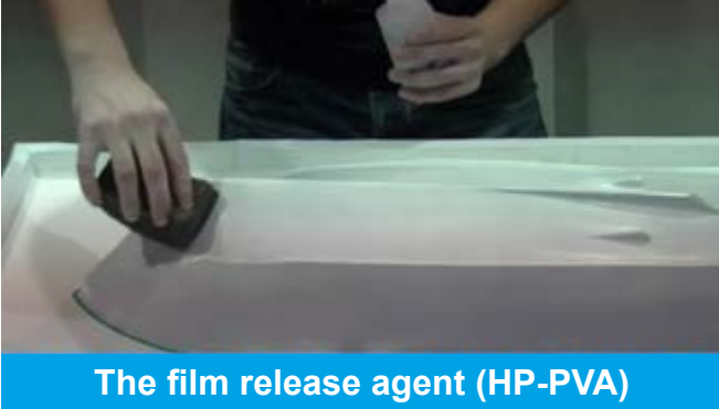
The film release agent is applied with a fine-pored sponge.
