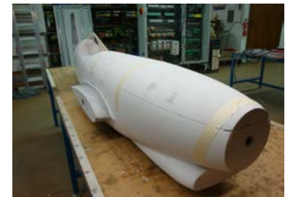
The model after it has been grinded and prepared for the moulding.
