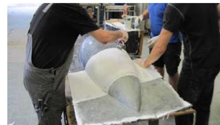
Reinforce back with epoxy resin and carbon/glass
