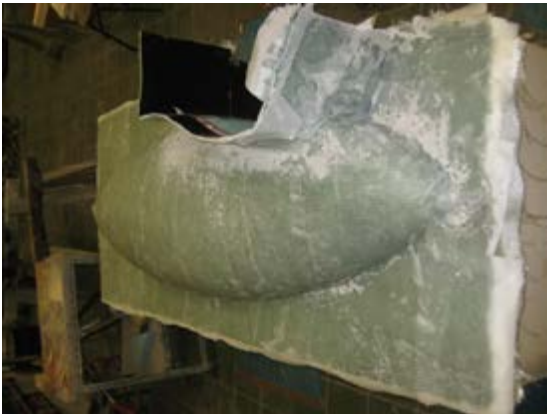
Epoxy resin & carbon/glass reinforcement
