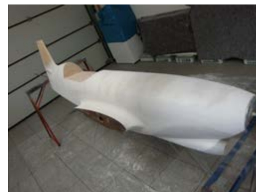
The model after it has been grinded and prepared for the moulding.
