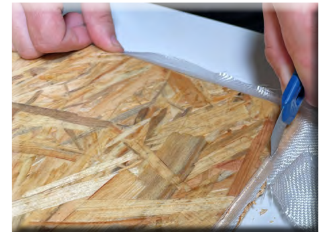
Excess glass fabric is cut off
