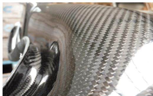
Abb. 34: In-Mould Coating transparent.
